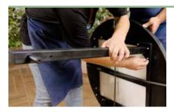
Place the wheel legs on the top side and tightened the screws by hand. The wheel shafts should face towards the outside.
