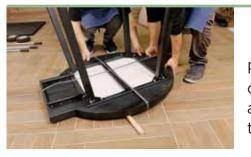
Put the wooden stick on a clean floor. Place the tray and feet upside down on the stick.
