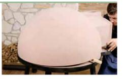
When the dome coincides with the recess of the base, lift slightly from the front, and remove the wooden stick.
