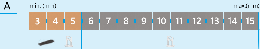
Spacer clips are used for all tiles with a thickness from 1/8" (3mm) up to 9/16" (15mm)
